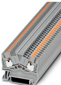
Feed-through terminal block, nom. voltage: 800 V, nominal current: 24 A, connection method: Push-in connection, 1 level, Rated cross section: 2.5 mm<sup>2</sup>, cross section: 0.14 mm<sup>2</sup> - 4 mm<sup>2</sup>, mounting type: NS 35/7,5, NS 35/15, color: gray
