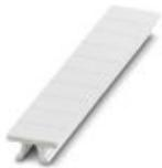
Zack marker strip, can be ordered: Strip, white, labeled according to customer specifications, mounting type: snap into tall marker groove, for terminal block width: 5.2 mm, lettering field size: 5.15 x 10.5 mm, Number of individual labels: 10
