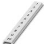
Zack Marker strip, flat, Strip, white, labeled, Printed vertically: consecutive numbers 1 ... 10, 11 ... 20, etc. up to 91 ... 100, mounting type: snap into flat marker groove, for terminal block width: 5 mm, lettering field size: 5.15 x 5.15 mm, Number of individual labels: 10
